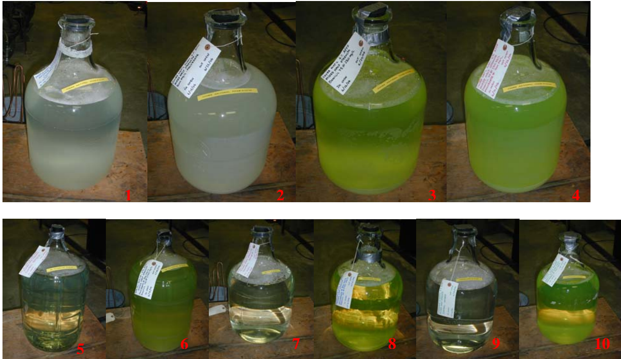
Figure 5. AFFF Solutions after Oven Aging for 10 Days. First row, from left to right: Sample 1, 2, 3, and 4 (National Foam). Second row, from left to right: Sample 5, 6, (3M); 7, 8 (Ansul); 9, 10 (Chemguard). The samples with the yellow-green color (3, 4, 6, 8, and 10) contain Dowicil.
