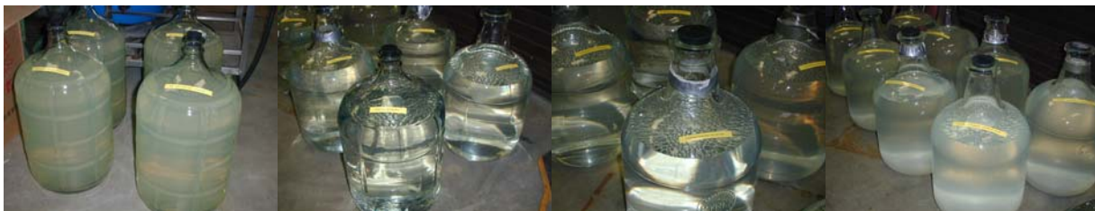
Figure 4. AFFF Solutions before Oven Aging. From left to right: 3M, Ansulite, Chemguard, and National.
