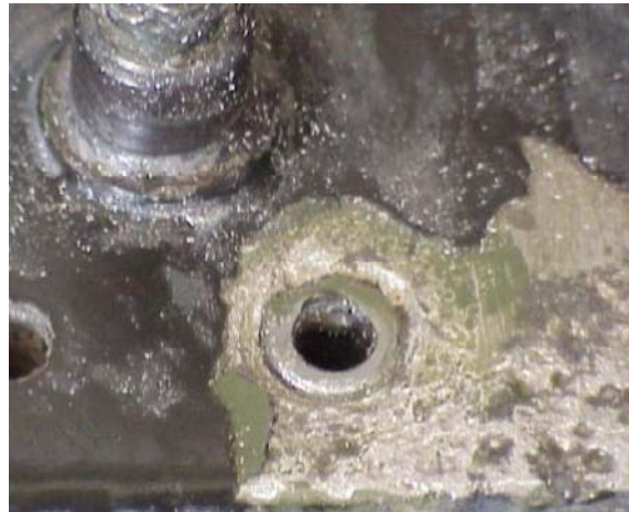
Figure 3. Corrosion around an insert on a helicopter Mg gearbox housing. (Courtesy Robert Kestler, FRC-E)
