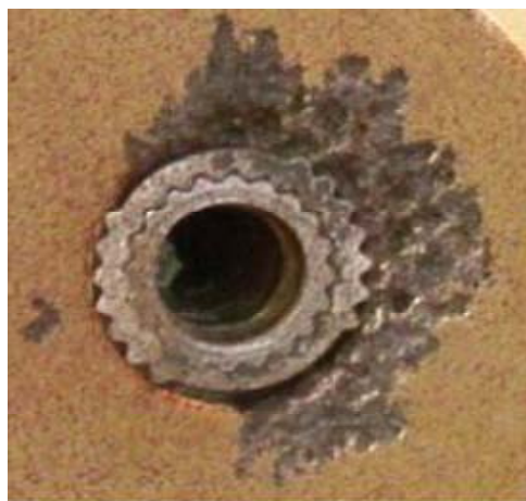
Figure 4. Rosan insert: corrosion around insert on a helicopter Mg gearbox housing (left) and cross section of insert with fitting (right). (Courtesy Robert Kestler, FRC-E)
