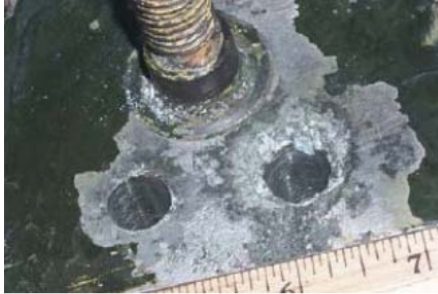
Figure 2. Corrosion around a stud and hole on a helicopter Mg gearbox housing. (Courtesy Robert Kestler, FRC-E)
