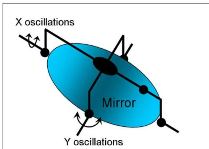
*Figure 1: One-mirror 2-axis design*
