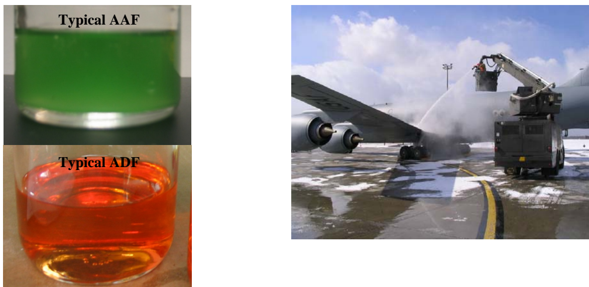
Figure 2. Typical Type I and IV Fluids and Spraying on Aircraft
