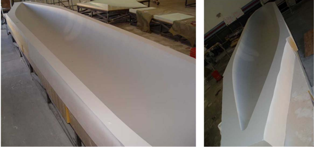
Figure 52 -C130 Sensor Pod Replica, Fabrication Tooling
