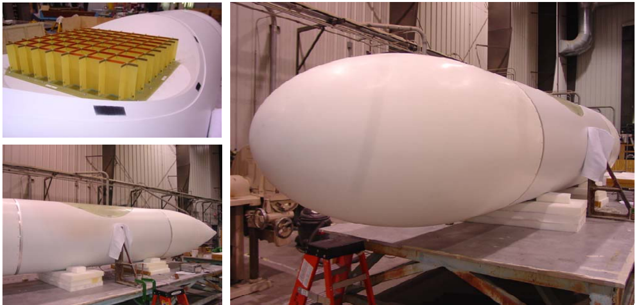
Figure 60 -FOPEN Meta-Array Integrated Assembly
