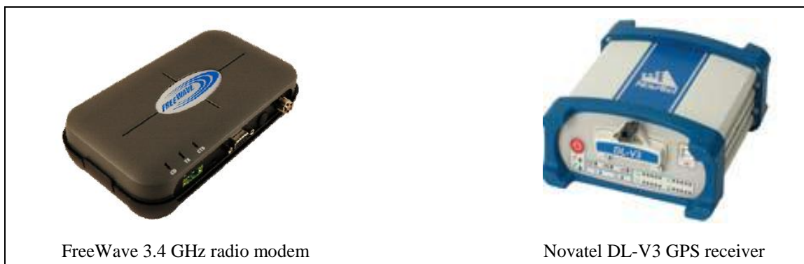
Figure 2. Photos of the radio and GPS receiver.
