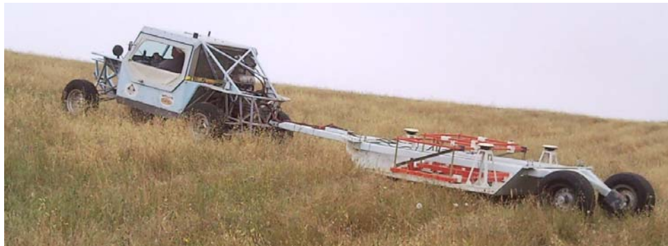
Figure 5-4 – MTADS EM61 MkII array pulled by the MTADS tow vehicle.
