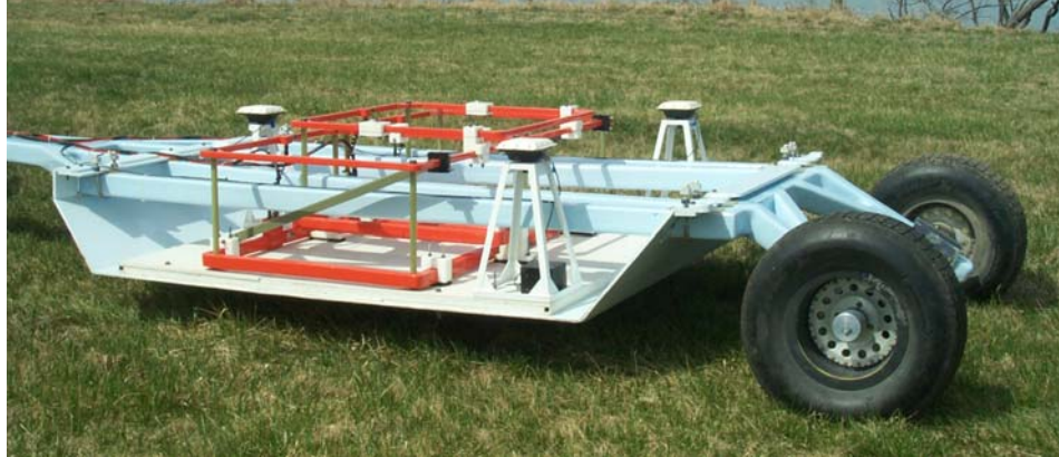
Figure 5-6 – Close-up of MTADS EM61 array with GPS and IMU.
