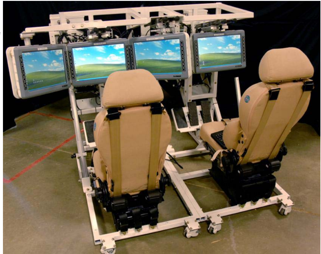
Figure: SCCS System Integration Lab (SIL). There is an identical SCCS in TARDEC's Crew Automation Testbed (CAT). The CAT is a M1126 ICV.
