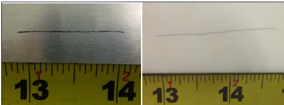
Figure 5. PRINT deposition on (left) polished aluminum sheet metal, and (right) aluminum oxide ceramic tile.
