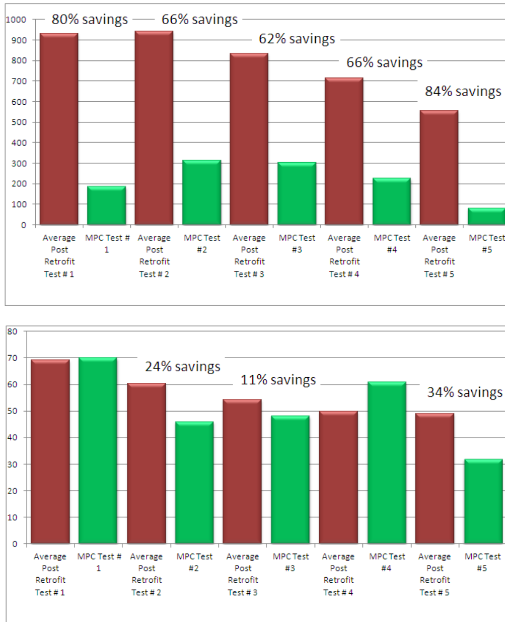
Figure 9. Summary of HVAC system energy use (top) and peak power consumption (bottom) measurements from final demonstration tests in February 2012.
