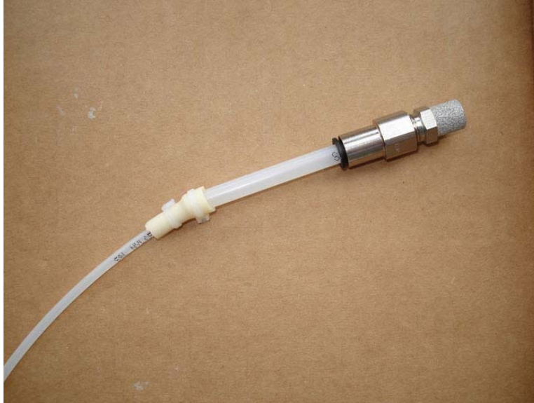
Photo 5.4.2: Example Soil Gas Sampling Implant
