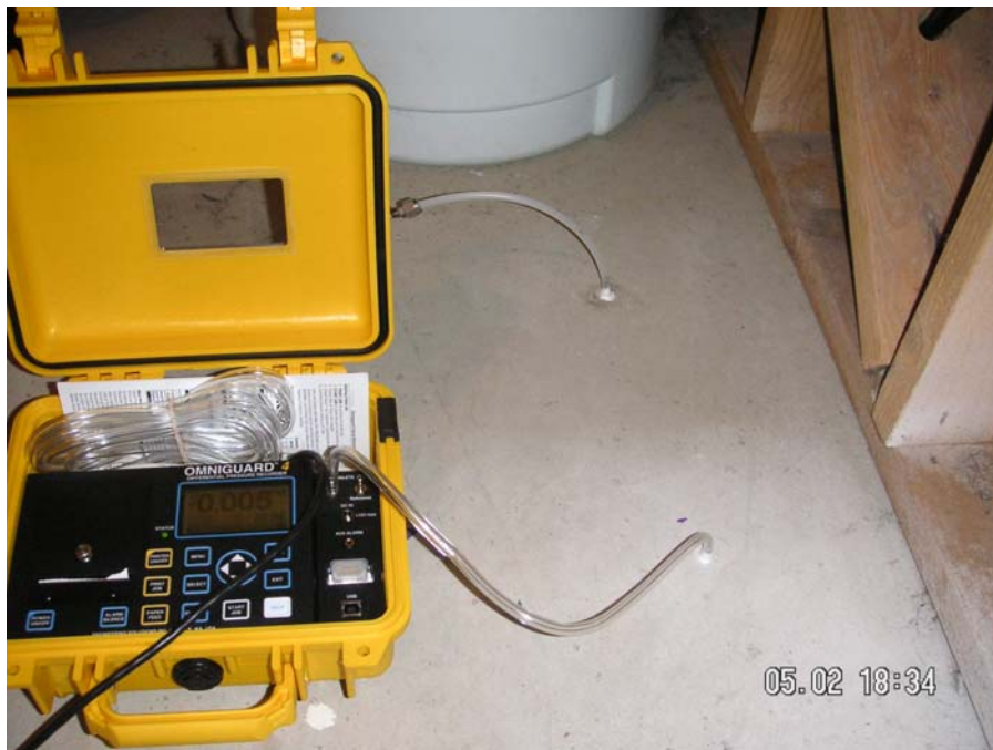
Photo 5.5.2: Pressure transducer installation
