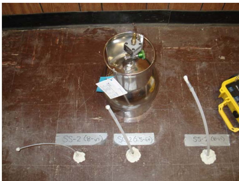
Photo 5.4.3: Example Sub-Slab Sample Port and Sample Train
