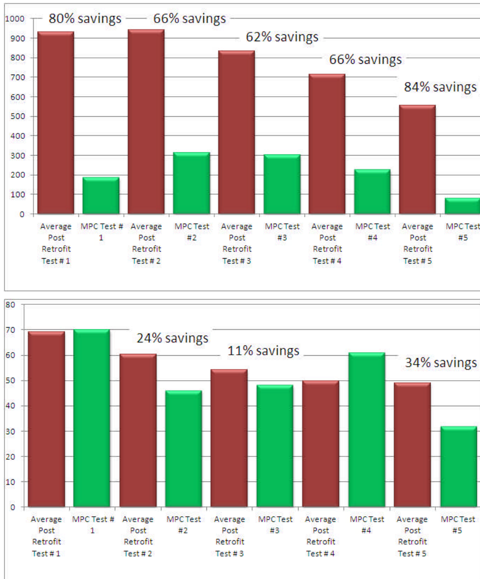
Figure 29. Summary of HVAC system energy use (top) and peak power consumption (bottom) measurements from final demonstration tests in Feb. 2012.
