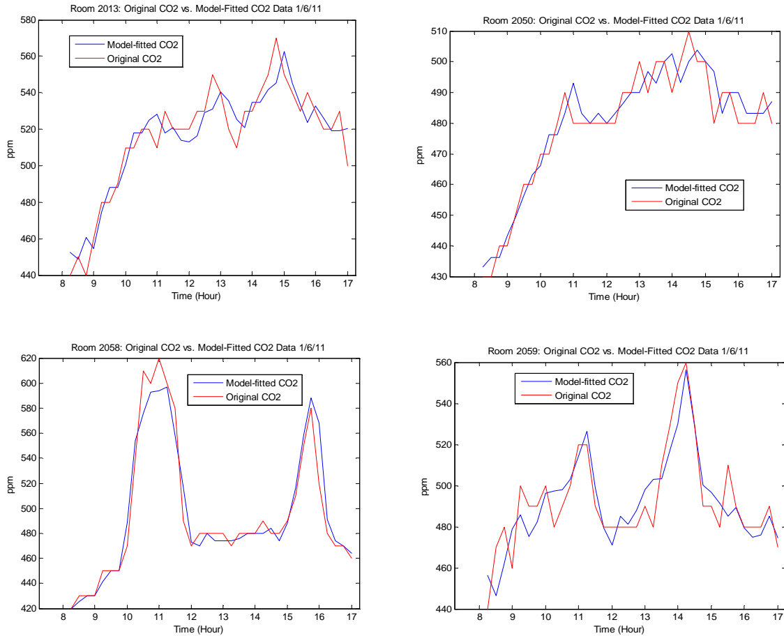
Figure 2.12 Comparison between measured and model predicted CO 2 levels.
