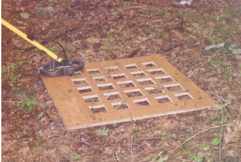
Figure 6-1: Template used to collect EM61HH array data during reacquisition.
