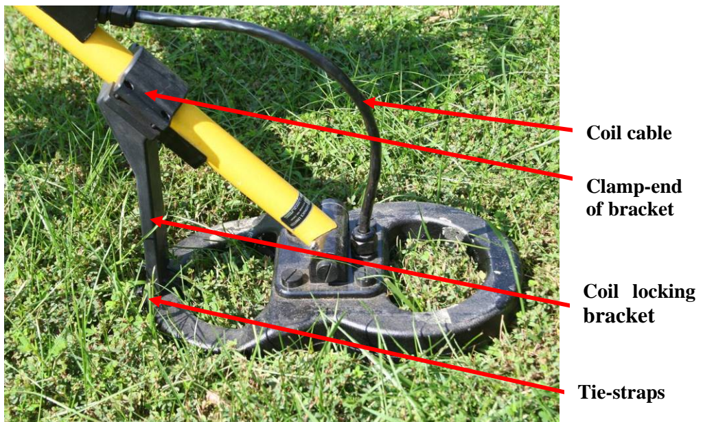
Figure A-6 The SAINT system coil-locking bracket
