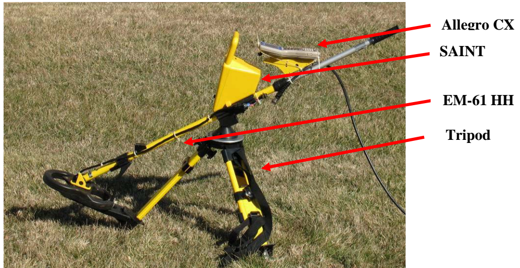
Figure A-1 The SAINT system installed on an EM-61 HH sensor
