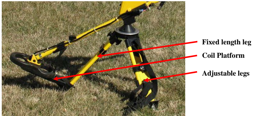
Figure A-5 The SAINT system tripod – leg details
