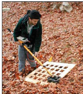
Figure 3-2 A standard approach to mitigating sensor positioning problem involves collecting data on a fixed grid over the target using a template laid on the ground. The sensor in the photograph is an EM61HH-MK2.
