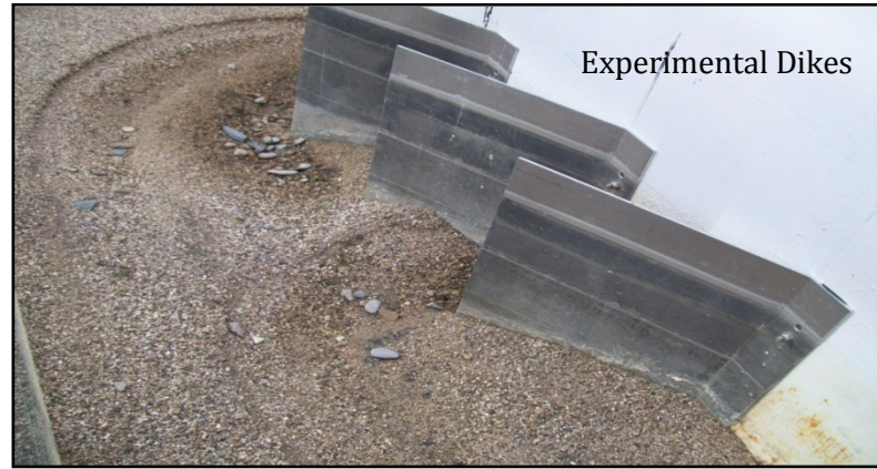
Fig.2b Picture of scoured bed
