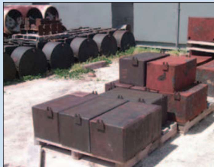
Thermally decontaminated (5X) ton containers, waste incineration containers, and metal boxes of tools to be barged from Johnston Island.
