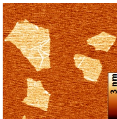
Fig 7: AFM height image of GO flakes on Si [5]
