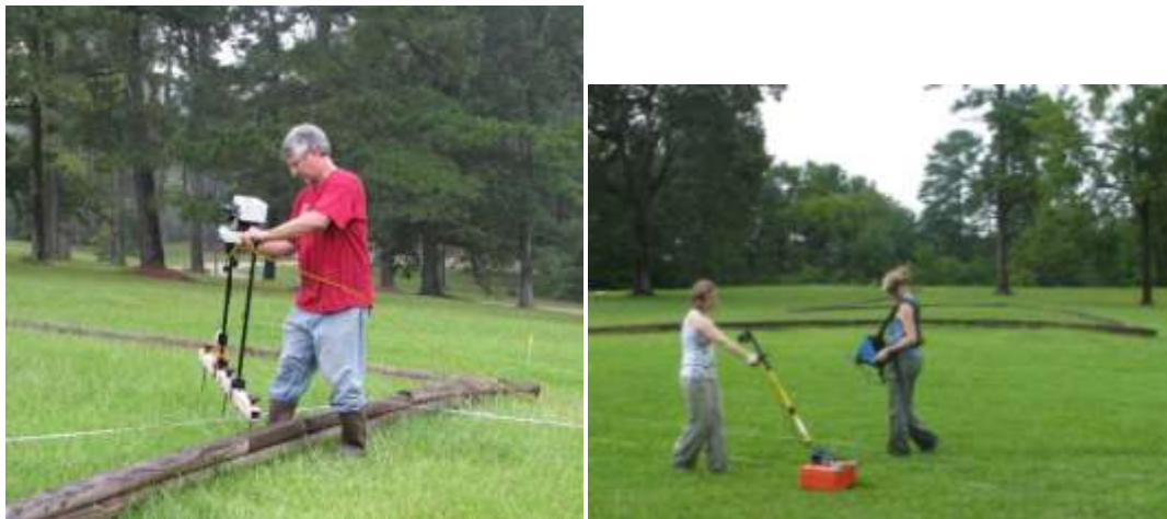
Figure 5-1: Preliminary survey of electrical resistivity (left) and GPR (right). Note the horizontal wood beams.
