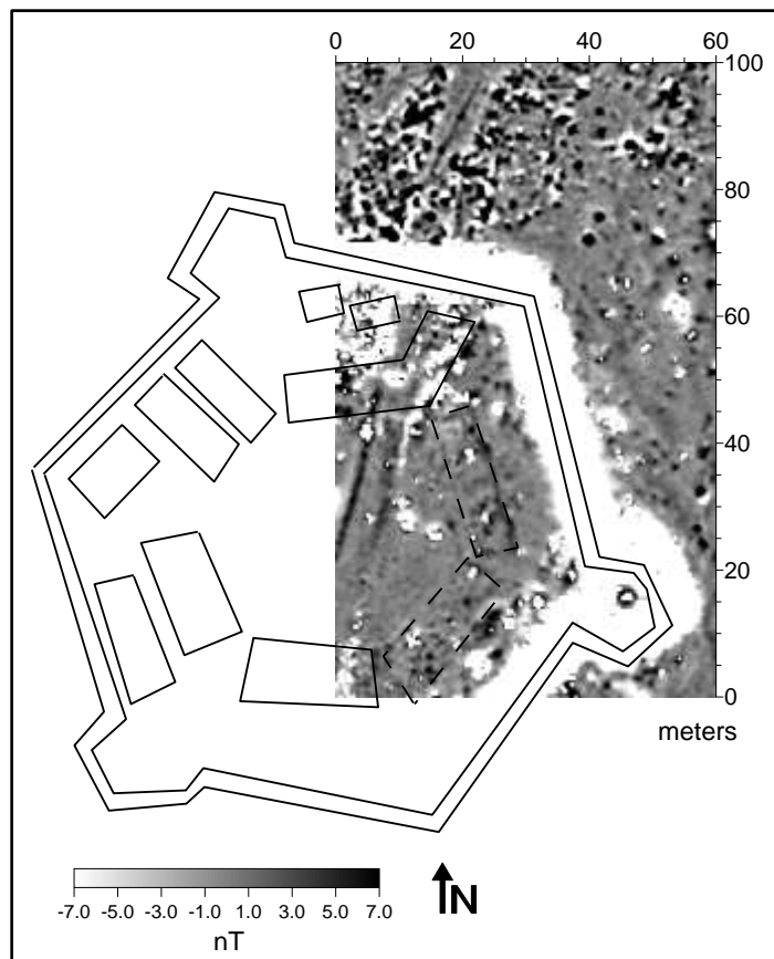
Figure 5-2: Magnetic gradient data collected during the preliminary survey atop outline of the 1767 map. The massive white anomaly is caused by iron rebar used to hold the horizontal wood beams in place.
