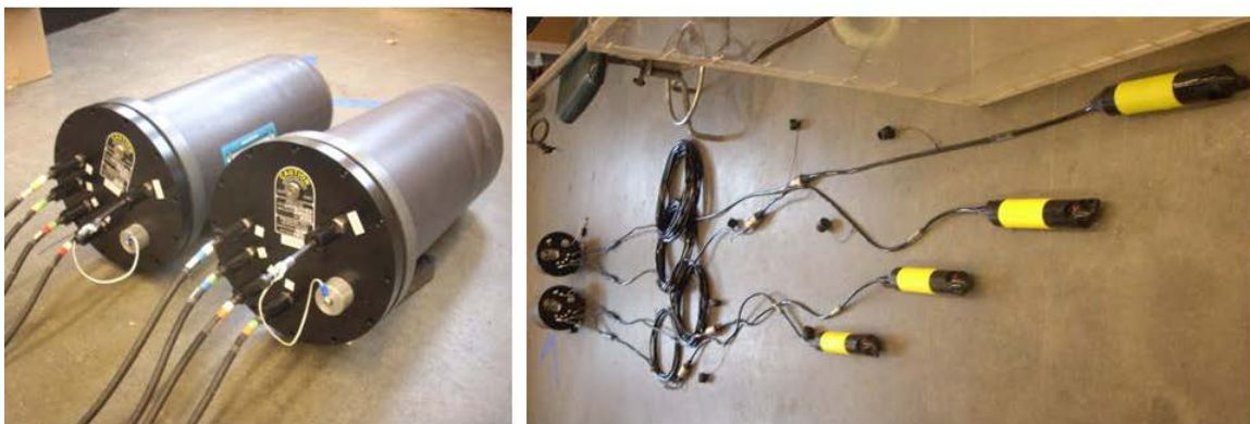
Figure 2. Left panel shows the two SHRU data collection systems. Right panel shows the geophone array consisting of gimbaled geophones.
