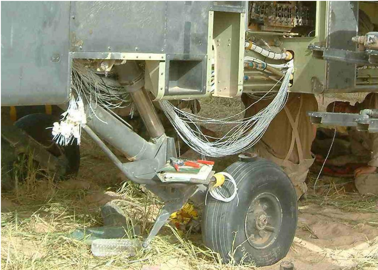
Figure 11: AH-64 Apache Electrical BDAR Damage and Repair
