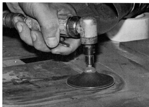
Figure 16: Machining of Scarf Joint with Disk Sander.
