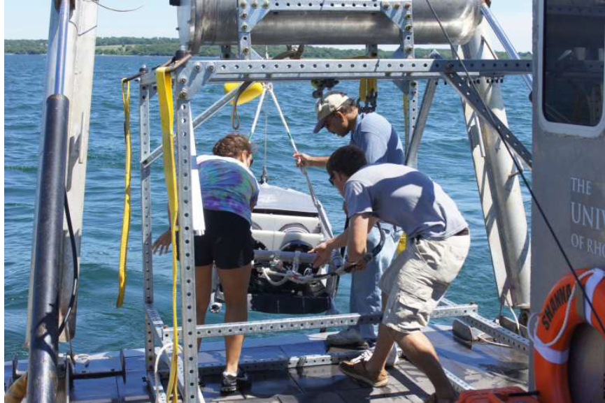
Fig. 9. Engineering test of URI geophone sled (being deployed) and the bottom mounted CSS (partially visible as frame) in Narragansett Bay, Rhode Island AUG 2011.
