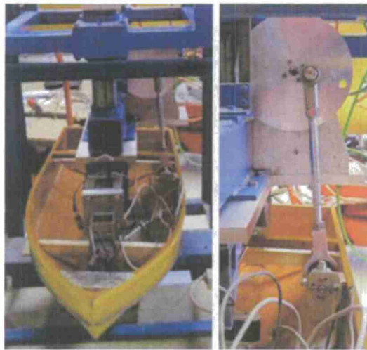
Figure 29. Images showing an overview of Forced Roll Mechanism and detail of the roll forcing design.
