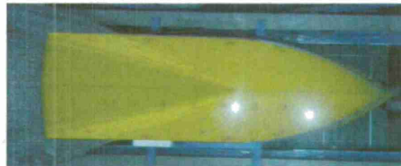
Figure 35. Underwater photograph of the model showing zero chine wetted lengths ( Fr_B=4.3 , zero roll angle).
