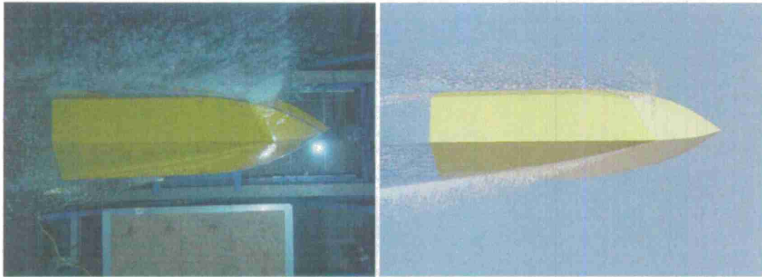
Figure 41. USNA underwater photograph (left) compared to NFA simulation (right); 20 degrees roll, U=20 ft/sec.
