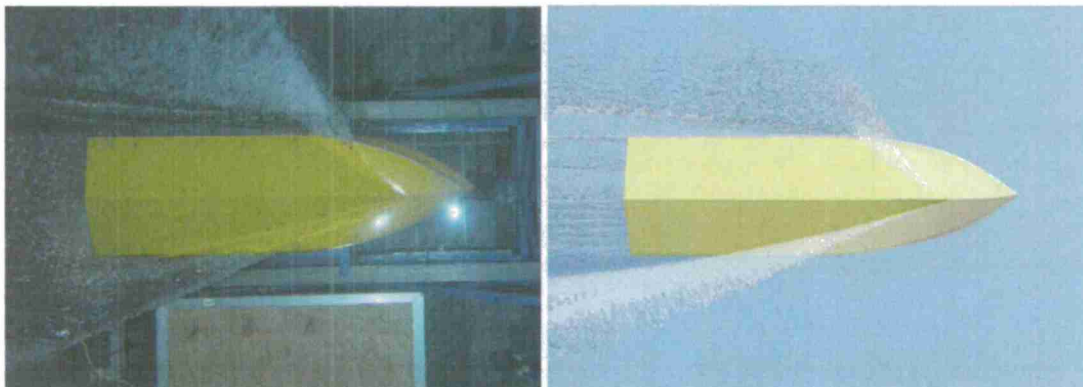
Figure 40. USNA underwater photograph (left) compared to NFA simulation (right); 10 degrees roll, U=20 ft/sec.
