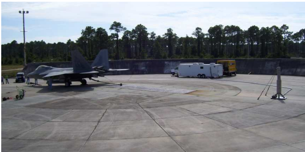
Figure 11-1. Trim pad and location of probe and instrument trailers with respect to aircraft
