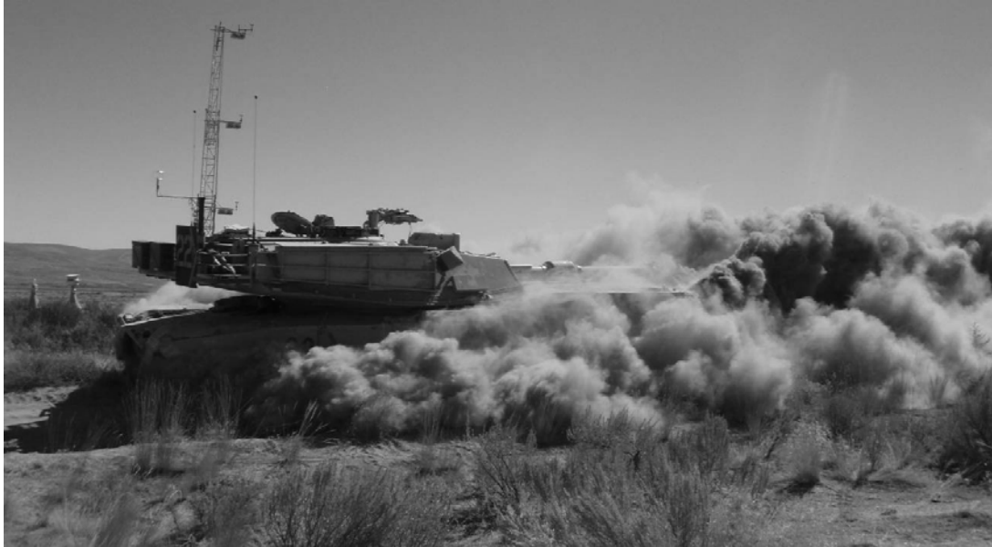
Figure 12. Image of M1A1 (Abrams) traveling at 40 km hr -1 on unpaved road at the YPG. Tower 1 is seen in the background along with PM 10 and PM 2.5 filter samplers. The vehicle is moving to the left of the image and the turret is pointing backwards.
