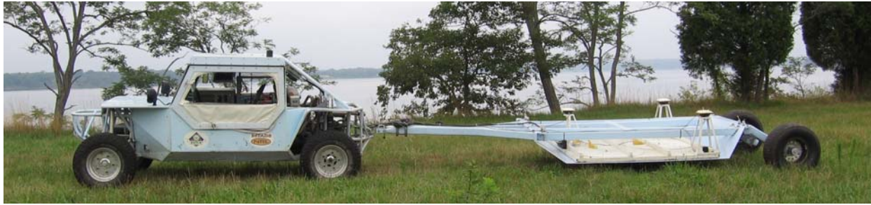
Figure 10. MTADS GEM-3 array in operation pulled by the MTADS tow vehicle.
