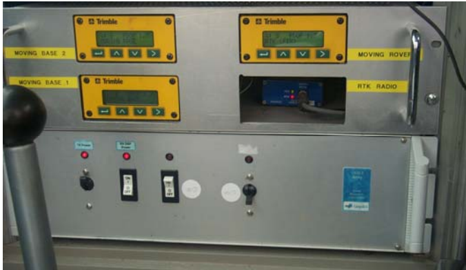
Figure 13. GEM-3 array control electronics and GPS receivers.
