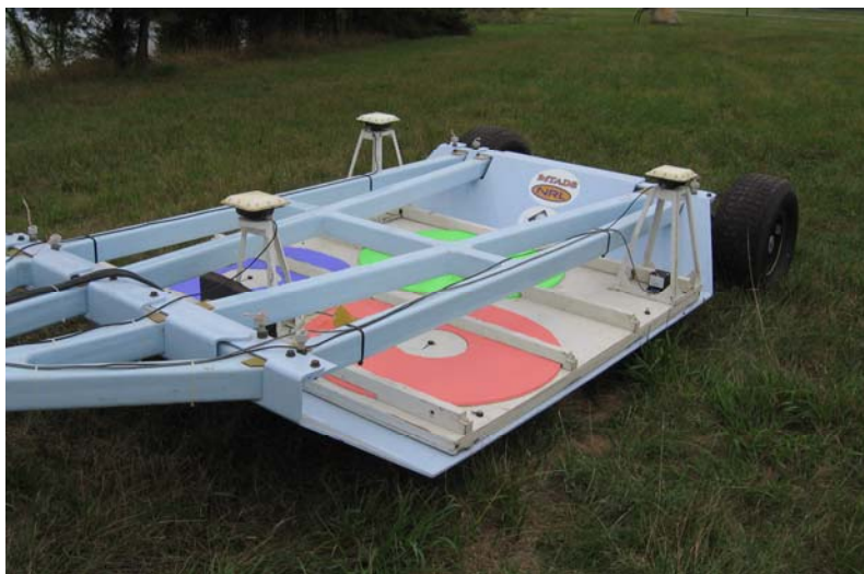
Figure 1. MTADS GEM-3 array mounted on the EM sensor trailer. Note the three GEM sensors, the three GPS antennae, and the IMU for platform motion measurement.
