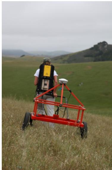
**Figure 3-4. EM61-MK2 CART collecting data at SLO.**
