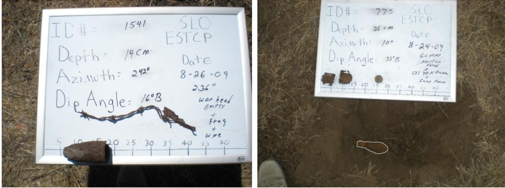
**Figure 5-17. Two commonly missed target are a 2.36-in rocket warhead collocated with a piece of barbed wire (left) and a 60-mm mortar with other munitions debris (right).**
