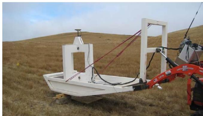
Figure 3-7. MetalMapper collecting data at SLO.
