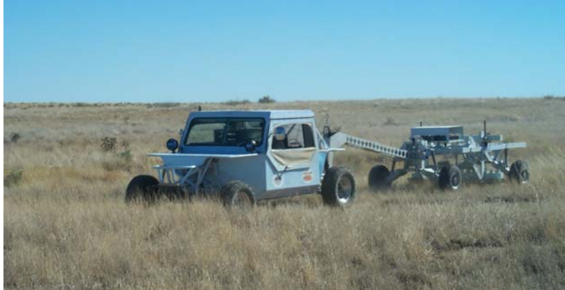
Figure 5-1 – MTADS tow vehicle and magnetometer array.
