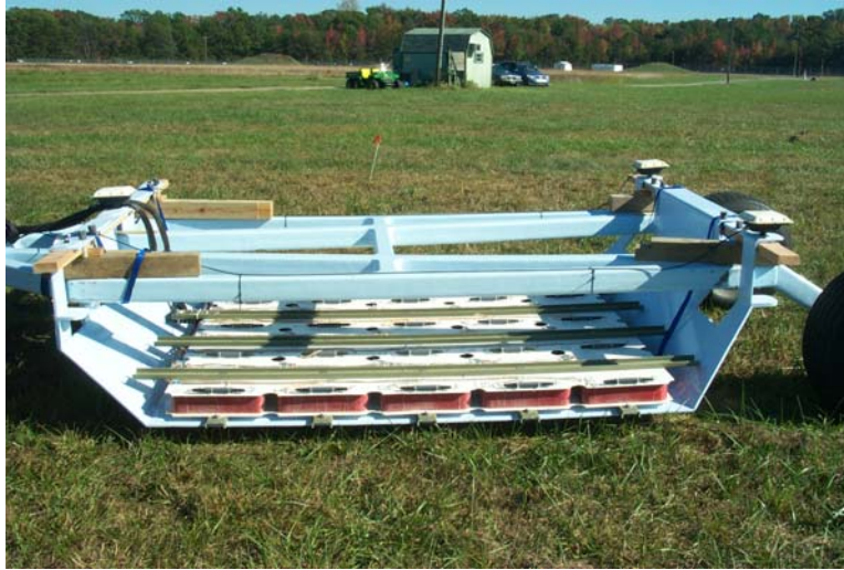
Figure 2-6 – Sensor array mounted on the MTADS EMI sensor platform.
