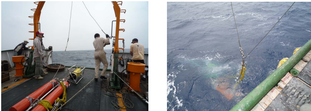
Fig. 3 The EAI 800Hz transducer and the pressure housings for the system and battery packages.
