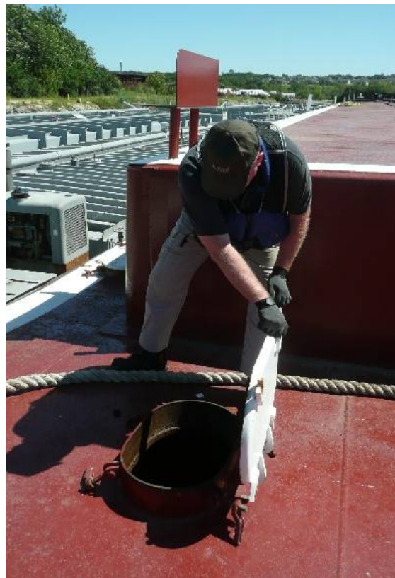
Figure C-3. Raised and flush hatch covers on rafted barges (Upper). Raised access hatch (lower).
