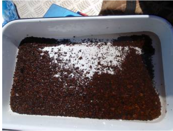
Figure 6. Example of material (mainly rust) pumped out of ballast tank during Trial 1.
