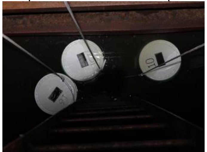
Cages suspended in ballast tank
