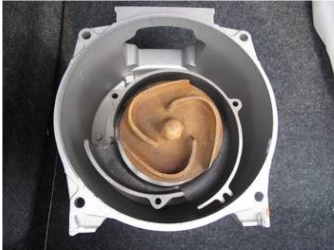
Impeller from 3-inch portable water pump
