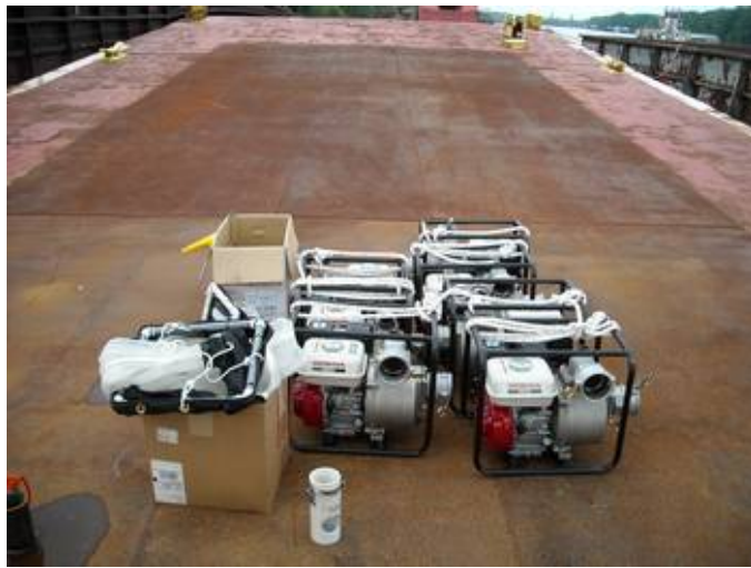
Pumps for emptying tanks
