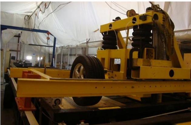
Fig. 7: Terramechanics rig carriage equipped with a pneumatic tire
