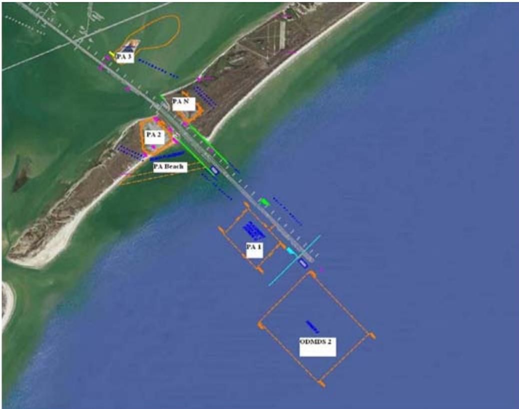
**Figure 8. Placement area locations (from PMP, Figure 7).**
