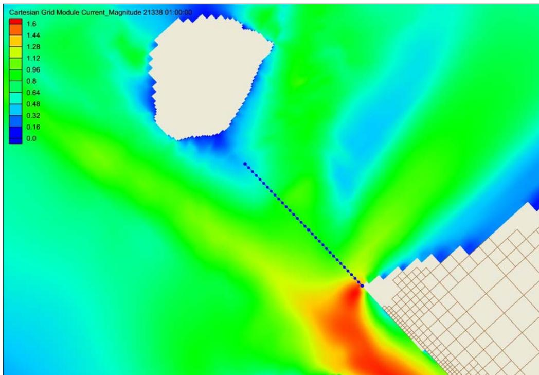
Figure 24. Line upon which the cross-current was determined.
