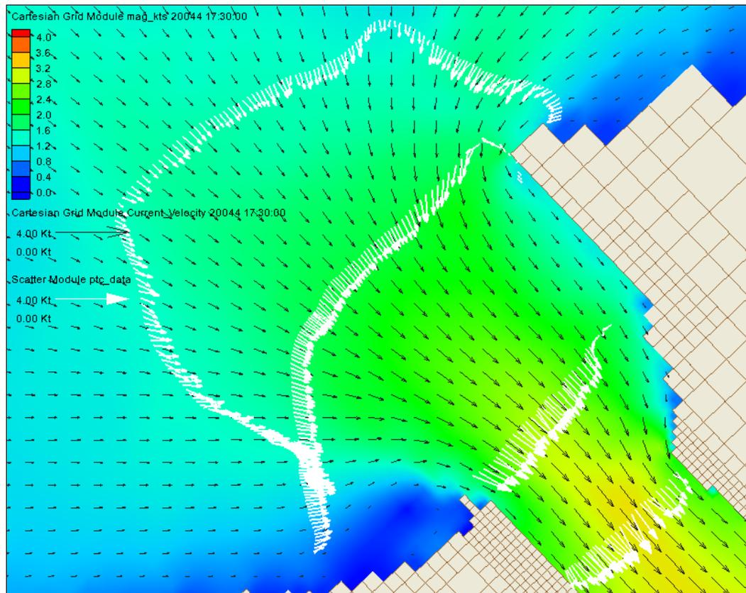
Figure 25. CMS calculated velocities (black arrows) compared with ADCP measured velocities (white arrows), 17 Nov 2004, 1730 GMT.
