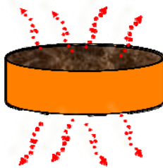
Figure C.1. Illustration of the physical system modeled showing an intact segment of porous media contained within a brass ring (5-cm diam. by 2.54-cm thick) with volatilization potentially occurring from the top and bottom exposed surfaces.
