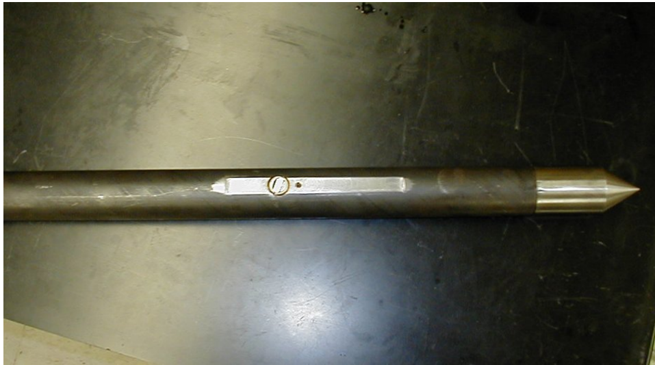
Figure 24. Completed dual-camera probe. The small hole to the right of the window is the set screw that holds the internal assembly in place.
