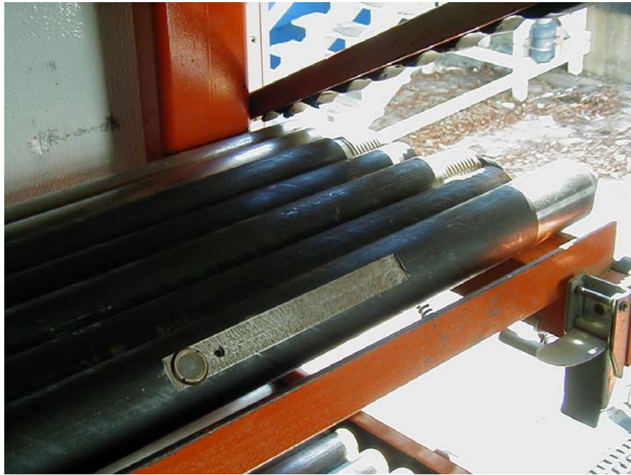
Figure 28. Probe on rack in SCAPS truck prior to field testing.
