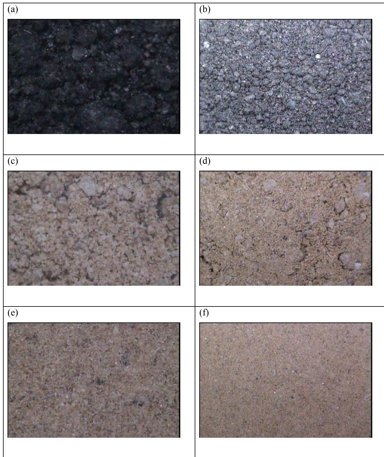
Figure 23. Digital images samples from the University of Arizona Soil Club used to test color resolution, (a) soil #7 at 1.6-mm field of view, (b) soil #7 at 6.4-mm field of view, (c) soil #15 at 1.6-mm field of view, (d) soil #15 at 6.4-mm field of view, (e) soil #1 at 1.6-mm field of view, (f) soil #1 at 6.4-mm field of view.
