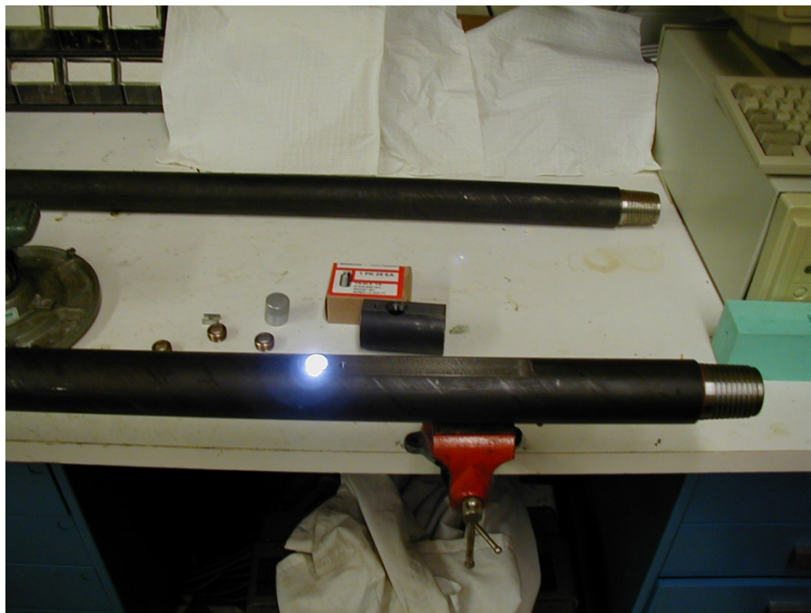
Figure 27. Completed video microscope probe inside of housing.
