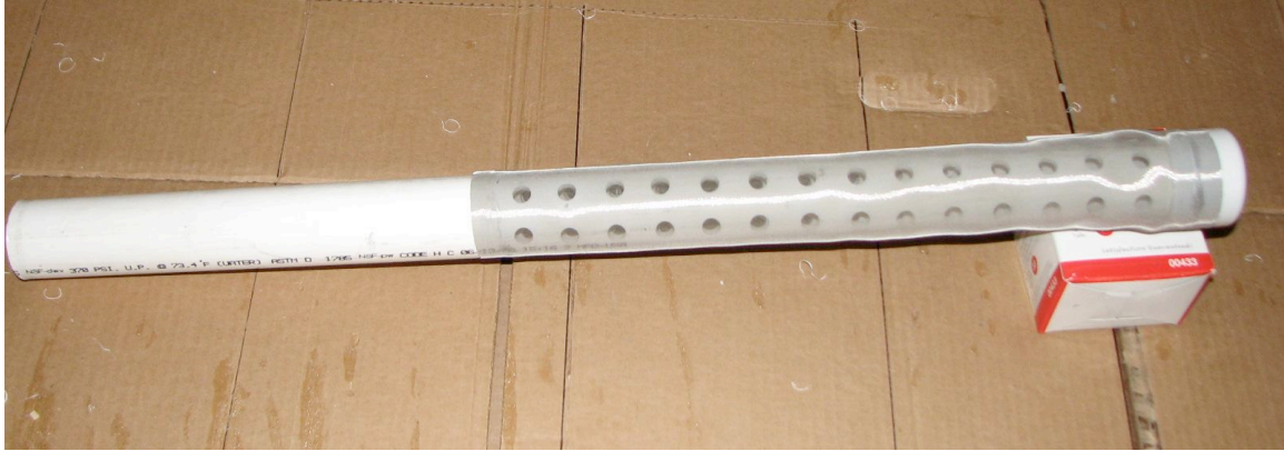
Figure 2: Construction of a synthetic aquifer well.
