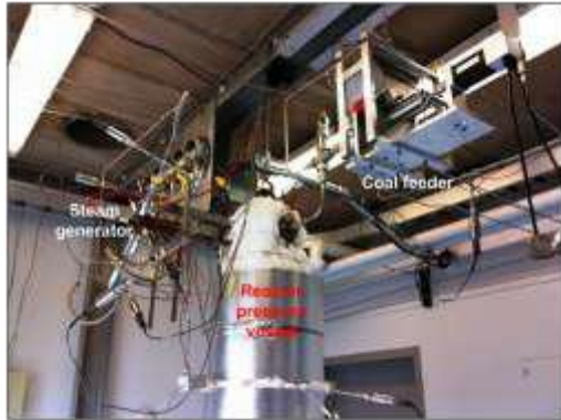
Figure 2.3: Gasifier reactor, hydrogen-oxygen steam generator and coal/biomass feeder in the test cell.
