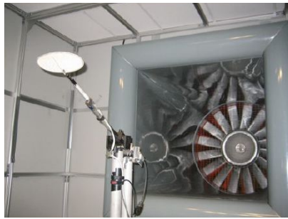
Figure 1. Installation of the wing in the wind tunnel. The model is mounted on the sting balance.
