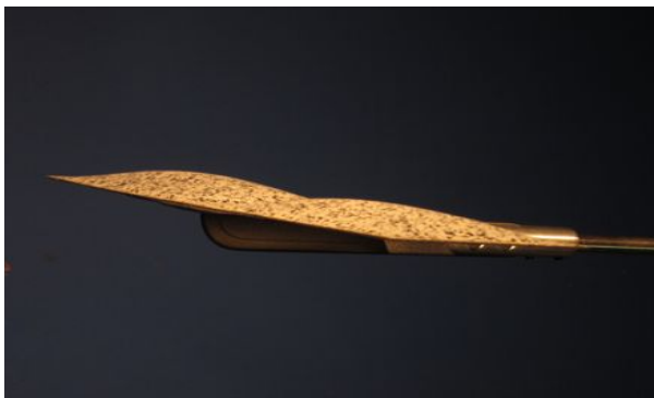
Figure 12. Speckled latex membrane wing during wind tunnel testing (left) and CAD model generated from the strain sensor surface reconstruction.
