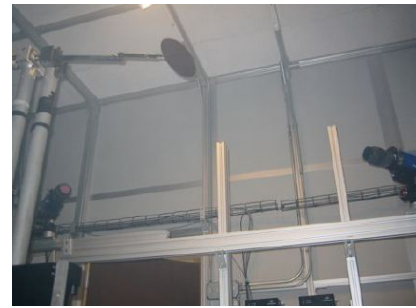
Figure 2. Installation of the wing in the wind tunnel. The PIV cameras are visible in the background.
