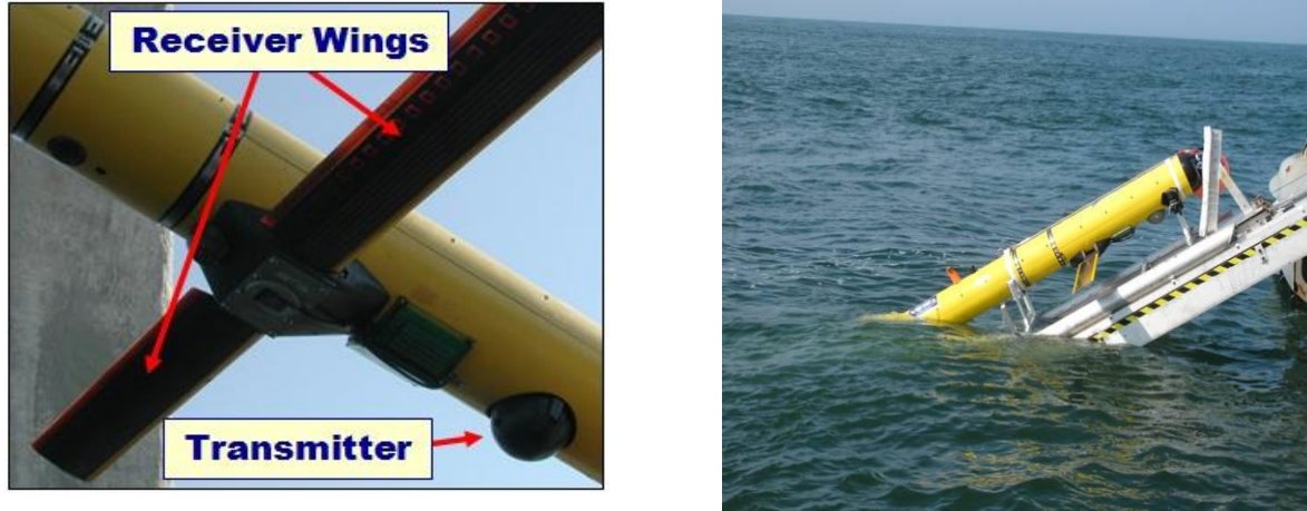
Figure 3. BOSS system as integrated on Bluefin 12 UUV: a) close-up of the BOSS receiver wings and transmitter and b) the Bluefin 12 UUV on the LRD system.
