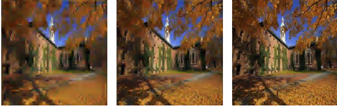
(a) Image obtained by using the 1% largest coefficients. (b) Image obtained by using the 3% largest coefficients. (c) Image obtained by using the 10% largest coefficients.
