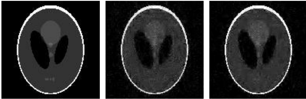
(a) Original 128 \times 128 phantom image. (b) BP: (SNR: 12.86dB). (c) NIHT: (SNR: 15.05dB).
