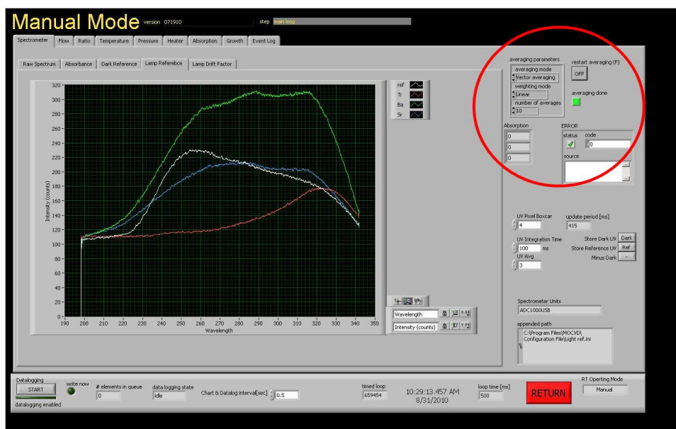
Figure 4: A screen shot of the RCC 2.0 showing signal averaging options (red circle) for processing the UV absorption
