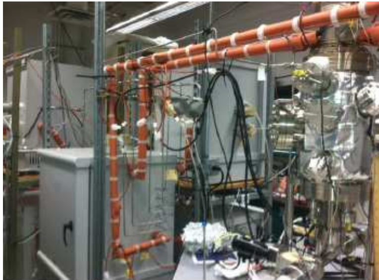
Figure 12: The ARL MOCVD reactor. Caltech and ARL worked together to transition MOCVD reactor technology from Caltech to ARL. The reactor design was based on the Caltech MOCVD reactor and was modified accordingly for additional complexity required by ARL. The reactor control software was developed jointly.
