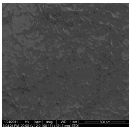
Figure 1. Scanning electron microscopy (SEM) picture of spray-deposited CNT on sapphire substrate.
