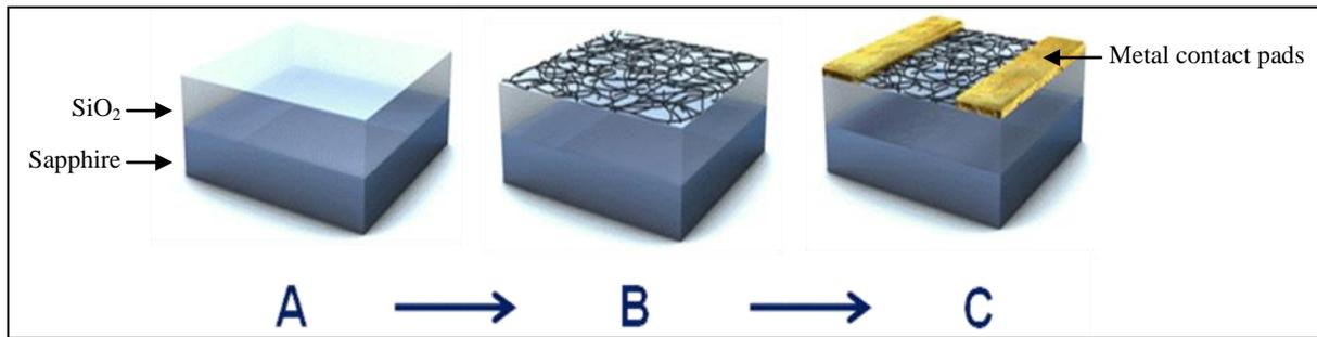
Figure 2. A schematic of the SWCNT fabrication process; (a) substrate template (sapphire/SiO<sub>2</sub>), (b) addition of SWCNTs, and (c) deposition of metal contact pads.
