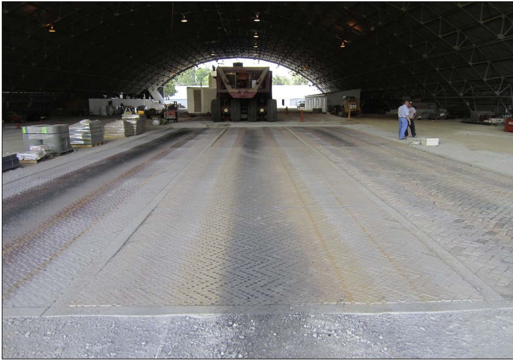
Figure 104. Test section after truck traffic.
