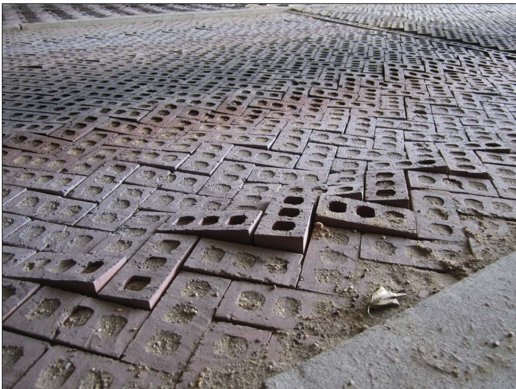
Figure 49. Item 3 wheel path at 10,010 passes of truck traffic.
