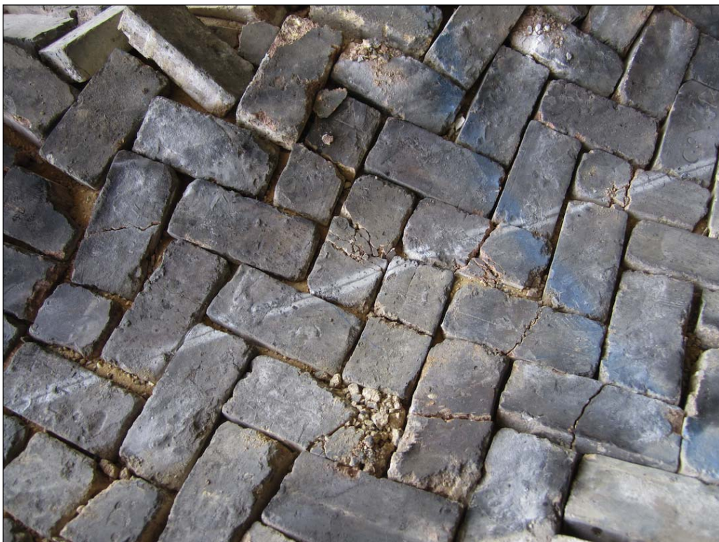
Figure 82. Center of wheel path of Item 2 at 44 passes of C-17 traffic.
