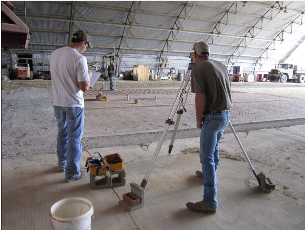
Figure 32. Longitudinal rod and level profile readings on Item 1.
