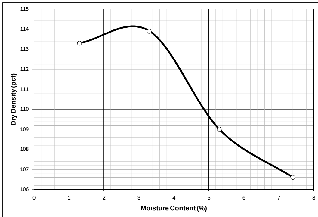
Figure 5. Dry density versus moisture content for blended GM base course.
