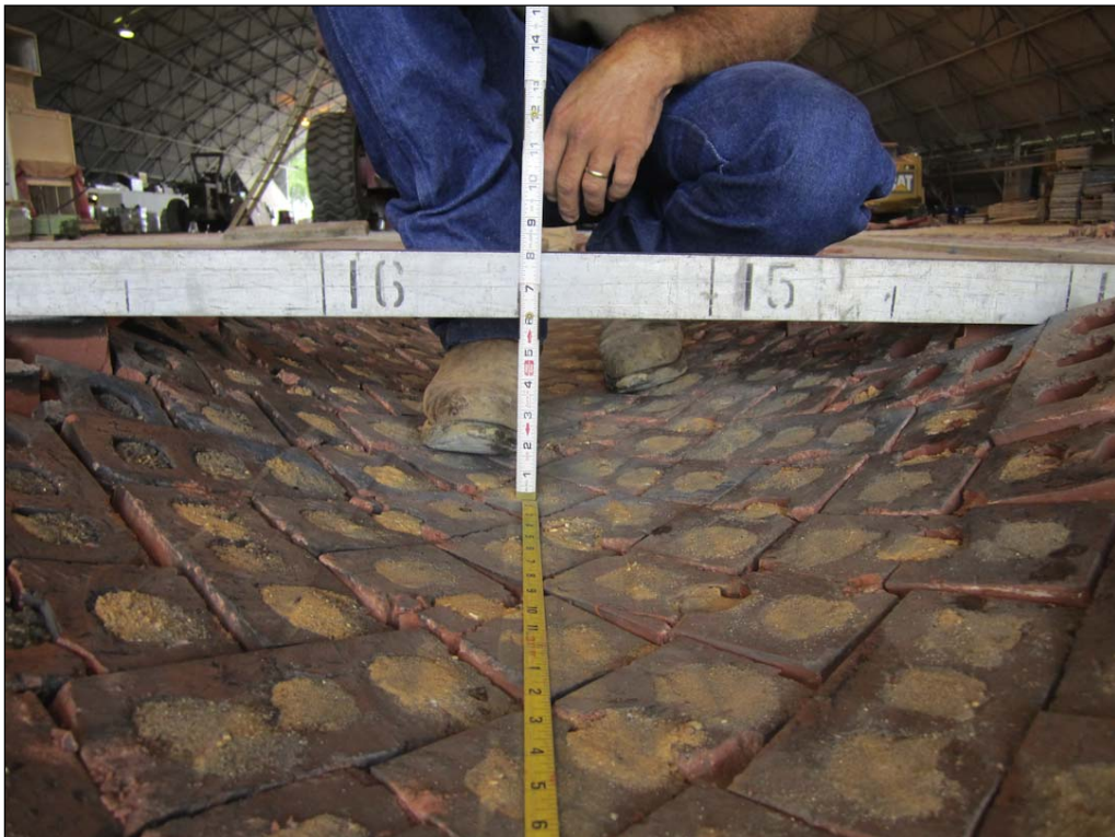
Figure 87. Item 3 rut depth measurement at Station 30 at 74 passes of C-17 traffic.
