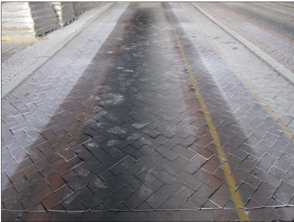
Figure 63. Item 5 overall view at 10,010 passes of truck traffic.
