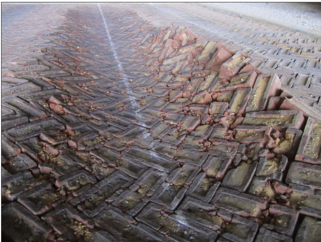
Figure 77. Item 1 wheel path at 88 passes of C-17 traffic.
