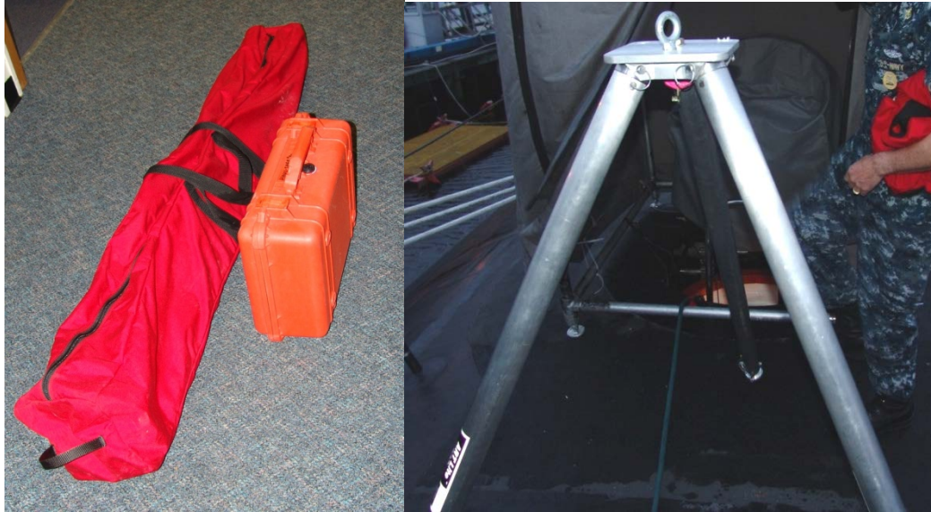
Figure 6. Haul-Safe Winch System (Spec Rescue International).
