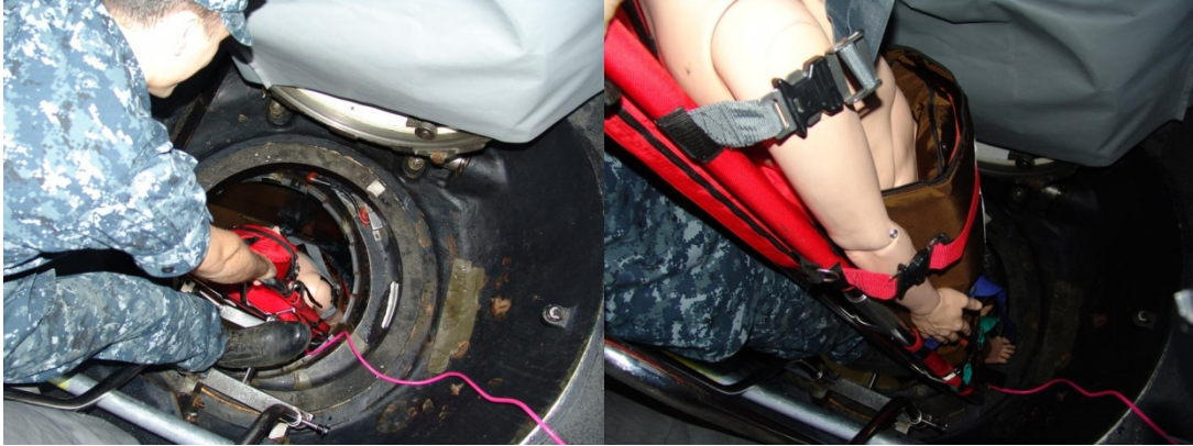
Figure 4. Extracting from the forward hatch with evident space constraints.
