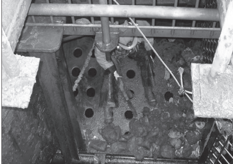
An observer cleans lumps of clay from the screen that strains dredged material.
