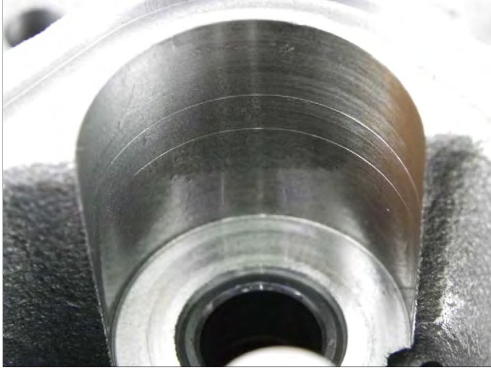
Figure E-10. Gear Pump Housing Wear
