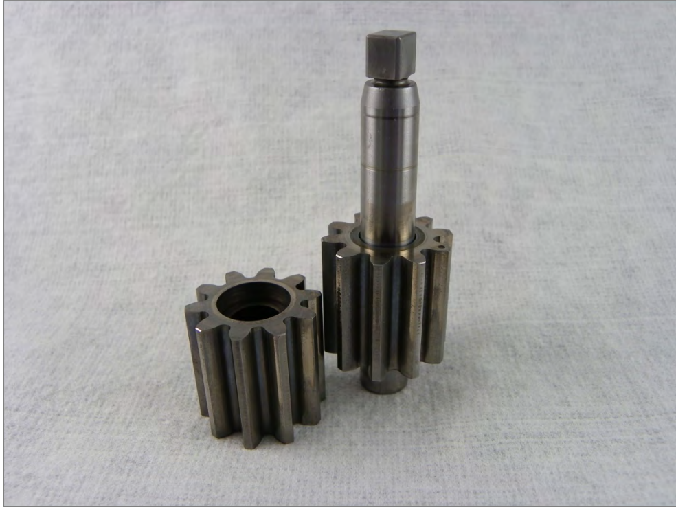
Figure F-12. Pump Gears
