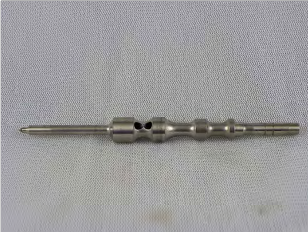
Figure C-25. Injector Needle (Failed)
