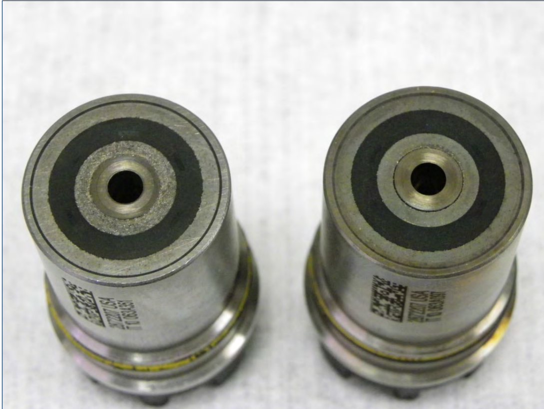
Figure 36. Solenoid Comparison – Suspected Failed (Left) and Typical (Right)
