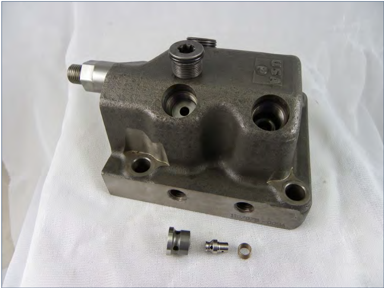
Figure 7. Inlet Check Valves
