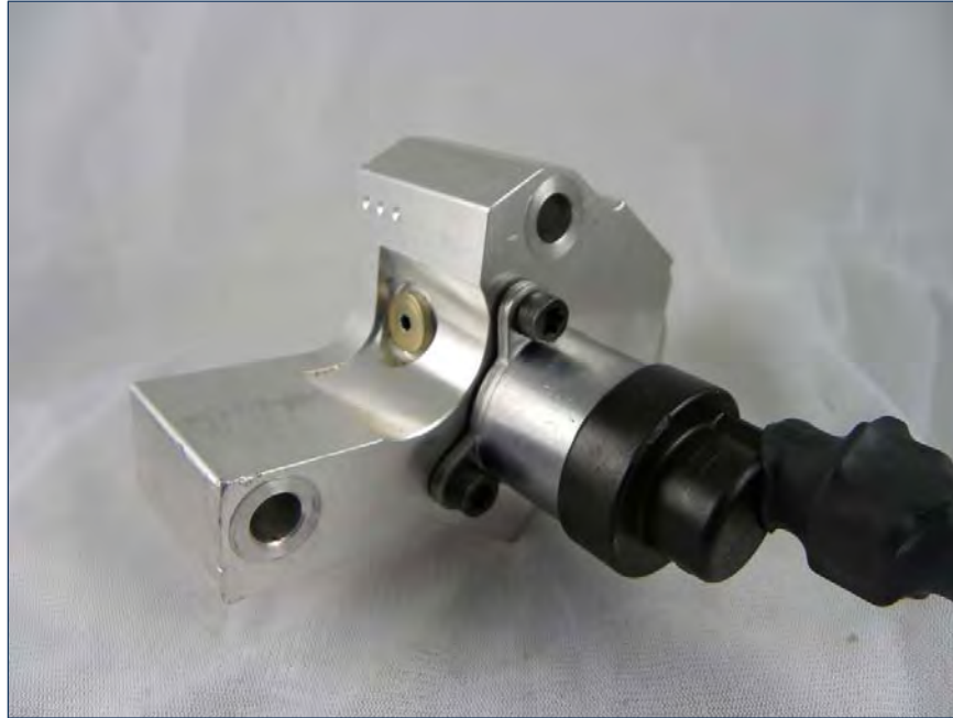
Figure 8. Control Manifold Portion of Pump
