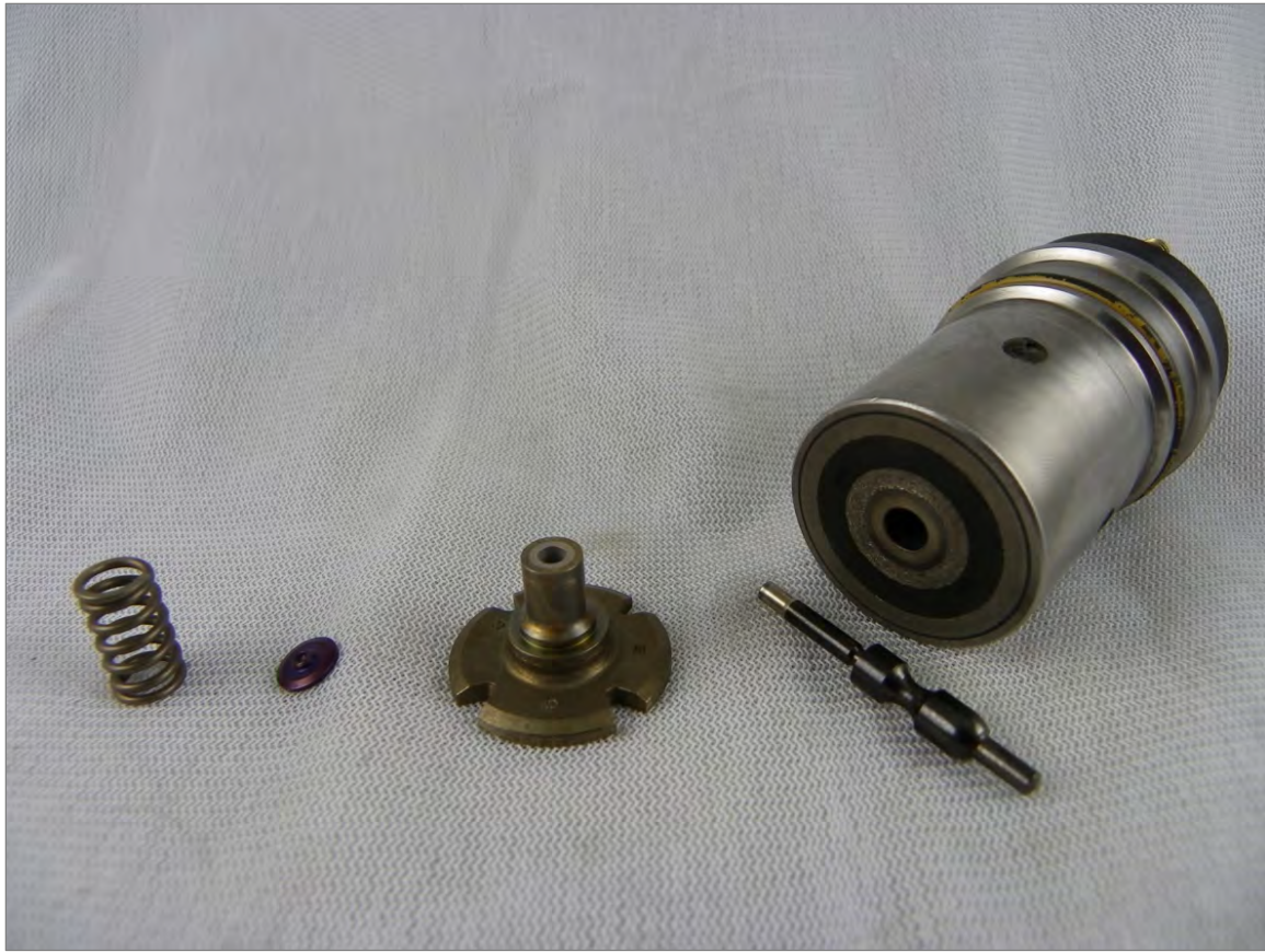
Figure C-15. Upper Injector Components (Failed)
