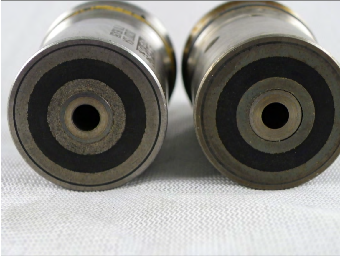
Figure C-16. Solenoid Units, Failed (Left) and Typical (Right)
