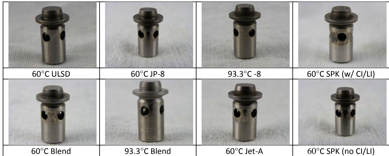
Figure 30. Pressure Relief Valve Side A
