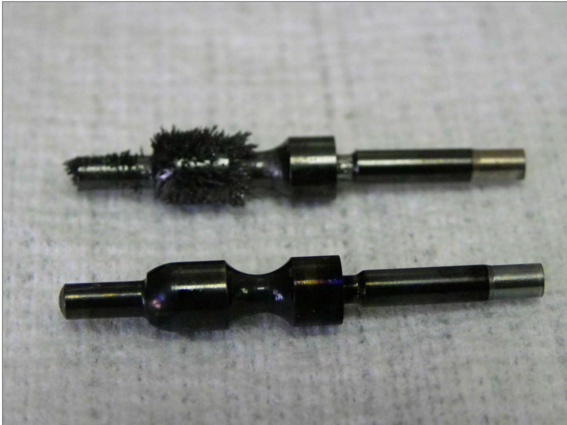
Figure C-17. Solenoid Plungers, Failed on Top, Typical Below
