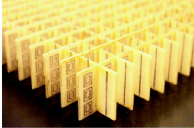
Figure 2. A negative-index MTM constructed using SRRs and wires embedded in fibreglass (From [3]).
