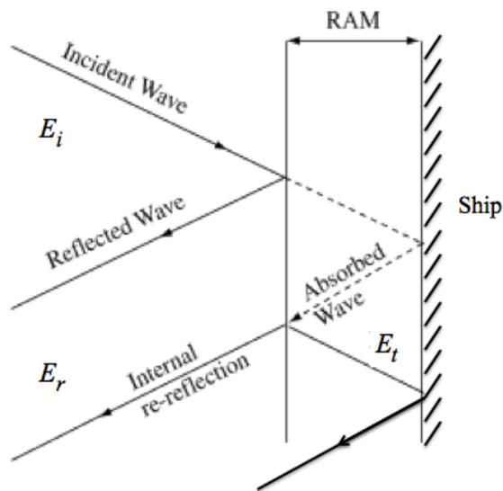
Figure 1. An illustration of how waves attenuate when RAM is applied (After [1]).
