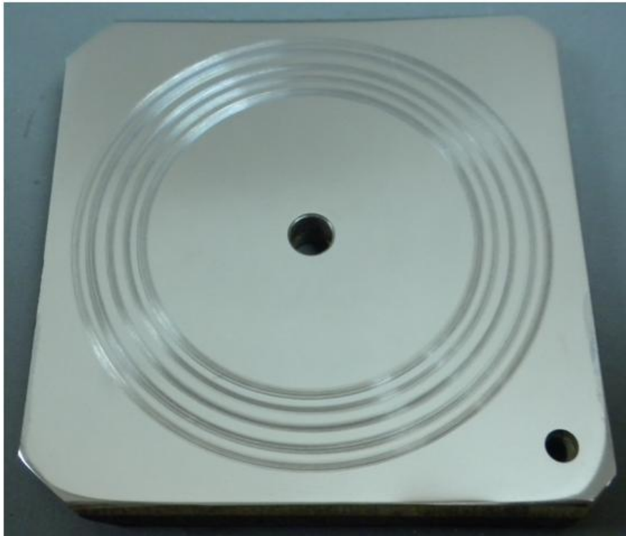
Figure 5.2. Polished 4140 Steel Sample after Ball-on-Disk Trials. (This figure is presented in color; the black and white reproduction may not be an accurate representation.)
