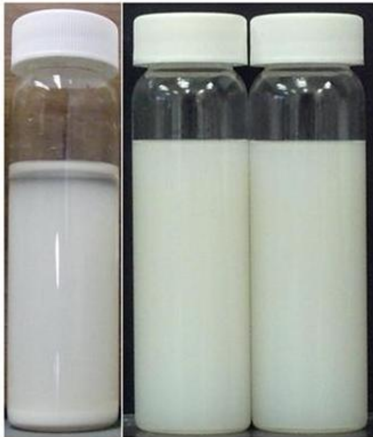
Figure 4.4. Oleic Acid Stabilized Nanofluid (Left) vs PIBSA stabilized nanofluids (Middle and Right) after Four Days. (This figure is presented in color; the black and white reproduction may not be an accurate representation.)
