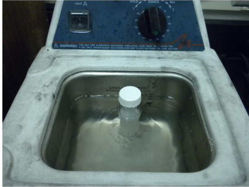
Figure 3.1. Branson 1510 Ultrasonic Cleaner Ultrasonicating an Alumina Nanofluid. (This figure is presented in color; the black and white reproduction may not be an accurate representation.)
