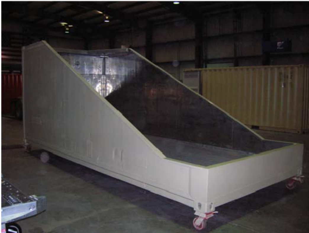
Figure 10. Completed field lysimeter prior to transport to the CAFB range.
