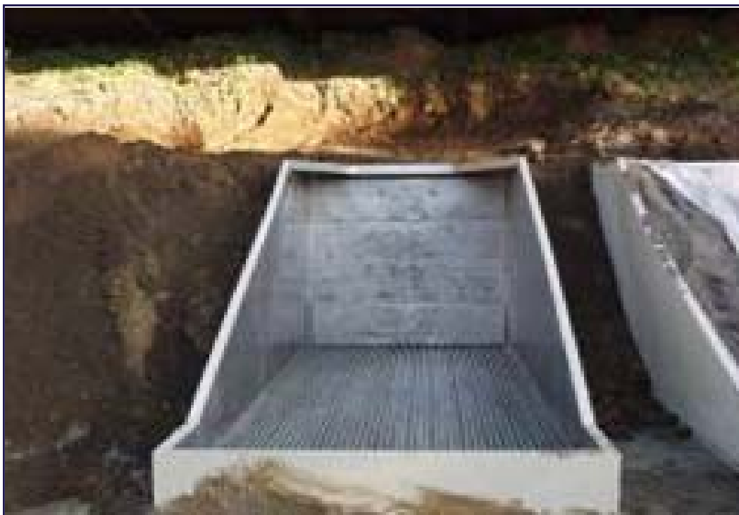
Figure 17. Placement of the three lysimeters in the impact berm in line with the three fixed firing positions.
