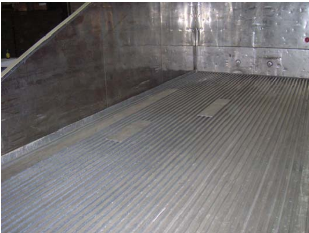
Figure 11. Interior view of the completed lysimeter demonstrating the ridged bottom to facilitate flow of the leachate from the amended ballistic sand.
