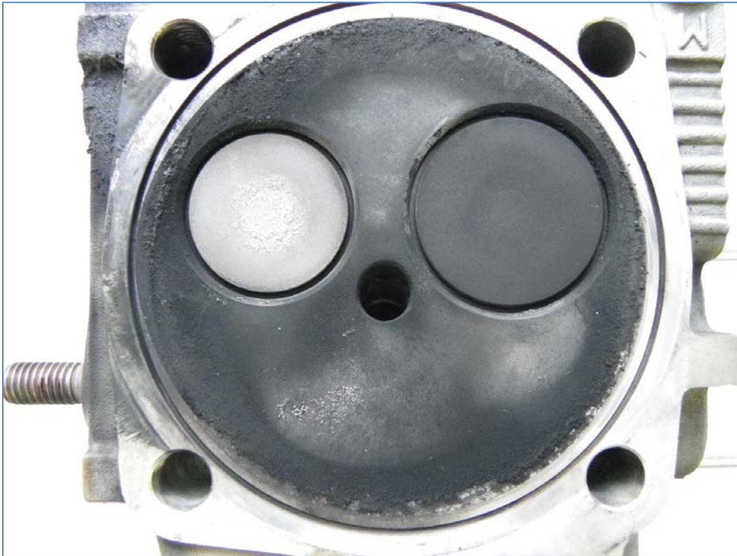
Figure 4. Cylinder head showing soot accumulation at gasket failure site on left side of picture
