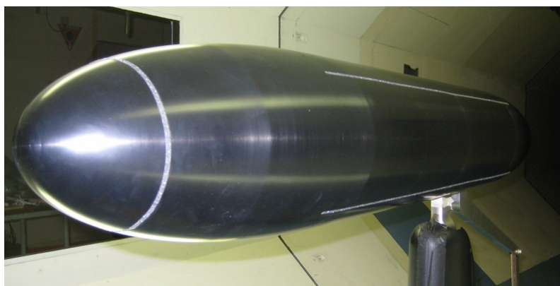
Figure 7 - Boundary layer transition strips attached longitudinally down the constant diameter section of the body
