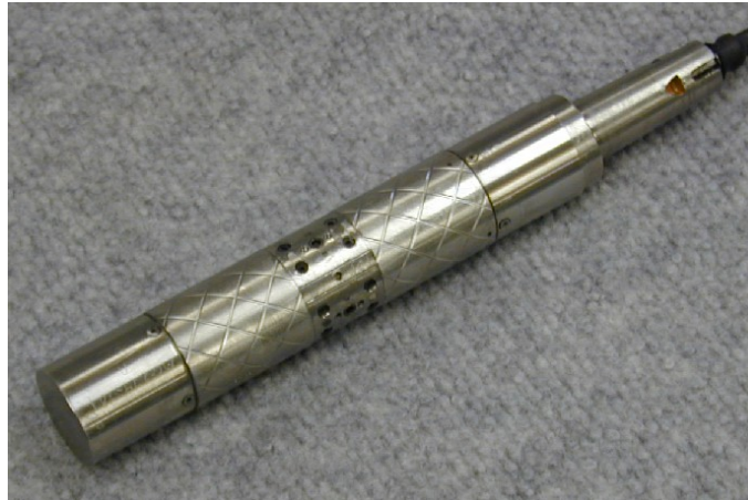
Figure 3 - Strain gauge balance DSTO-BAL-04
