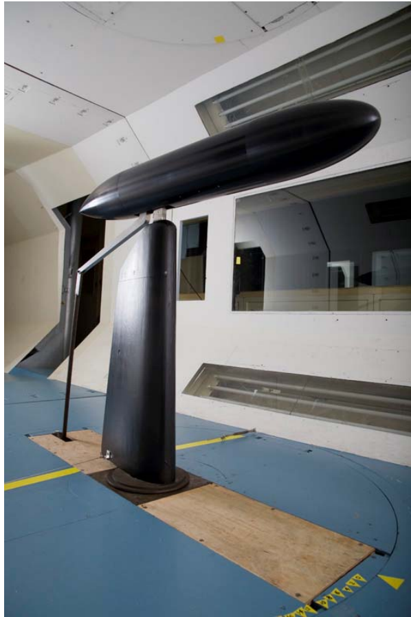
Figure 1 - Generic submarine model mounted in the DSTO low speed wind tunnel
