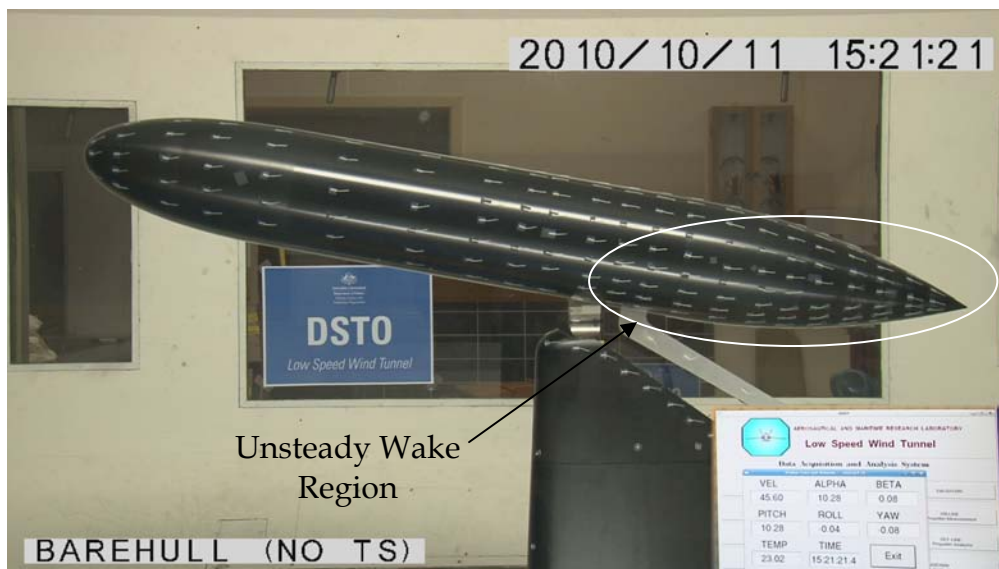
Figure 9 - A typical tufting flow visualisation result showing unsteady flow over the aft-body of the model at high-incidence
