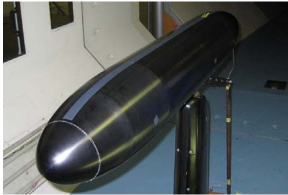
Figure 6 - Boundary layer transition strip attached circumferentially at 5% of its body length ( l )
