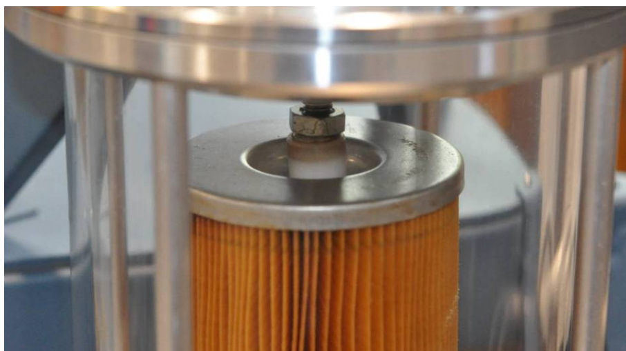
Figure 28: Top of T56 ESF in the FC290 showing the Wash Housing plunger bearing directly onto the solid top of the filter element.
