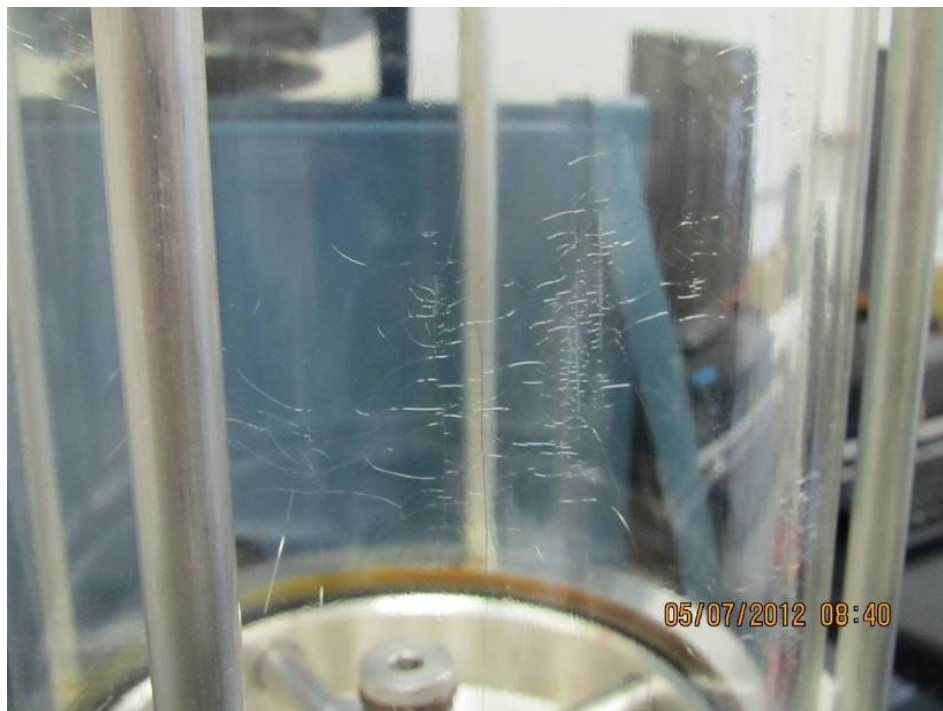
Figure 34: Wash Housing showing crazing
