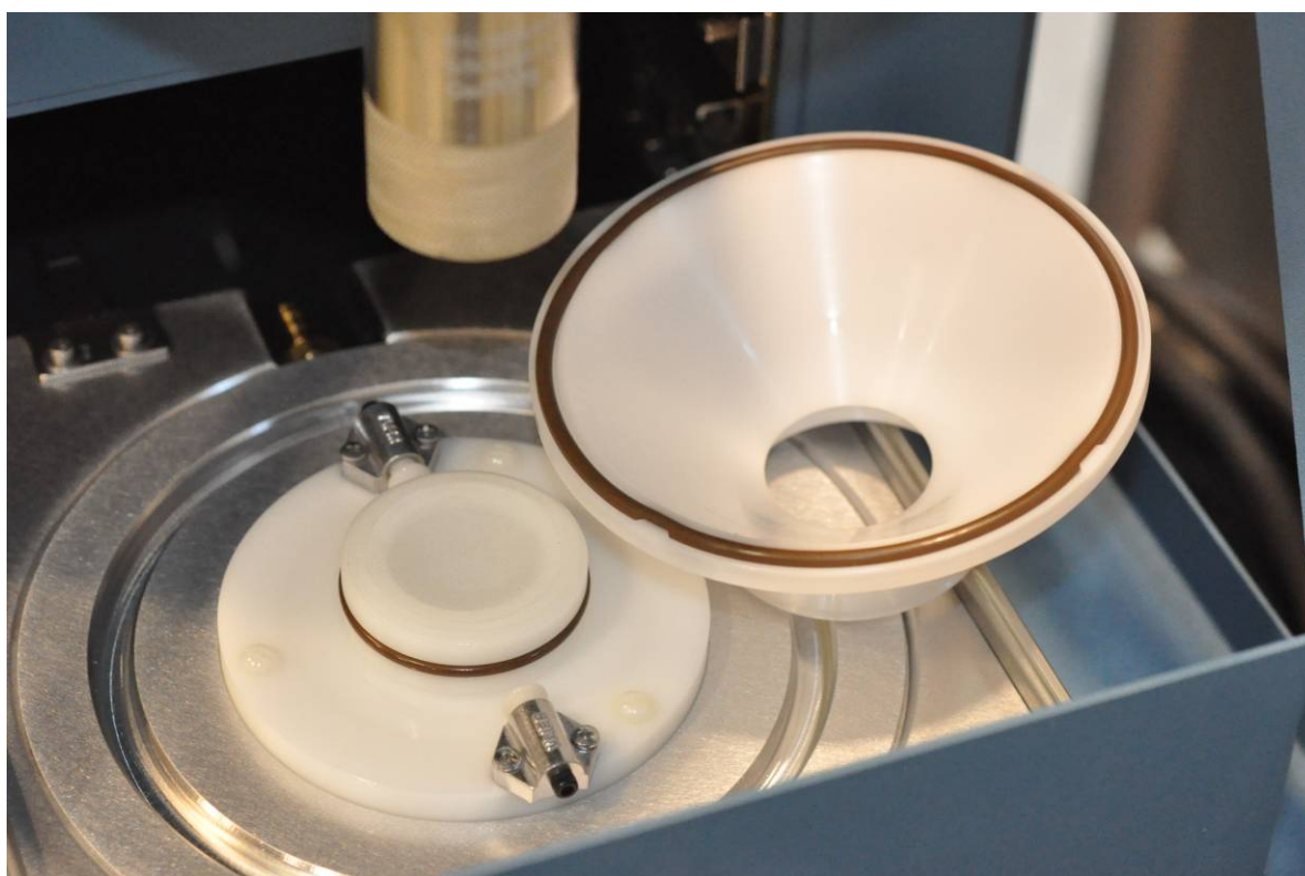
Figure 24: Sample filter patch holder as delivered.
