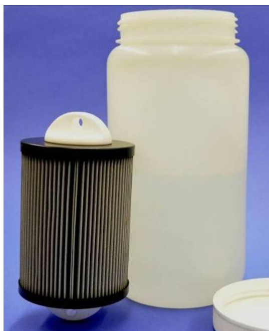
Figure 4: Plugged F117 oil filter and extraction container
